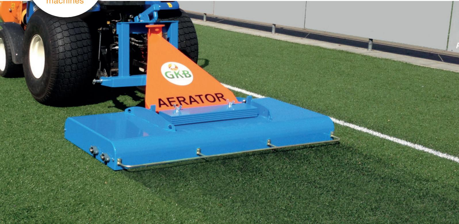
THE GKB AERATOR HAS BEEN DEVELOPED FOR THE DECOMPACTION AND AERATION OF ARTIFICIAL TURF ON WHICH SAND AND/OR RUBBER INFILL IS USED. THE INFILL MATERIAL IS COMPACTED WITH EACH USE OF THE PLAYING SURFACE, WHICH LEADS TO LOSS OF QUALITY IN TERMS OF BOUNCE, CUSHIONING AND WATER DRAINAGE. THE AERATOR COMBATS THIS COMPACTION, REGENERATING THE PLAYING SURFACE'S TECHNICAL CHARACTERISTICS.
