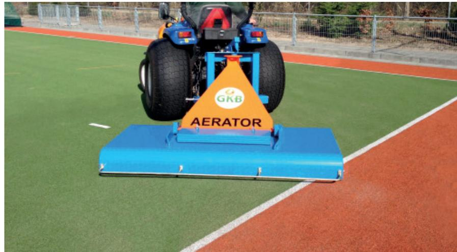
THE HINGED FRAME ENSURES THAT THE AERATOR ALSO WORKS WELL AROUND TURNS, WHICH MAKES IT VERY USER-FRIENDLY AND EFFICIENT. THE MACHINE IS PLACED IN AND OUT OF OPERATION BY PUTTING THE WHEELS, IN WORK OR TRANSPORT POSITION WITH OF A LEVER SYSTEM.
