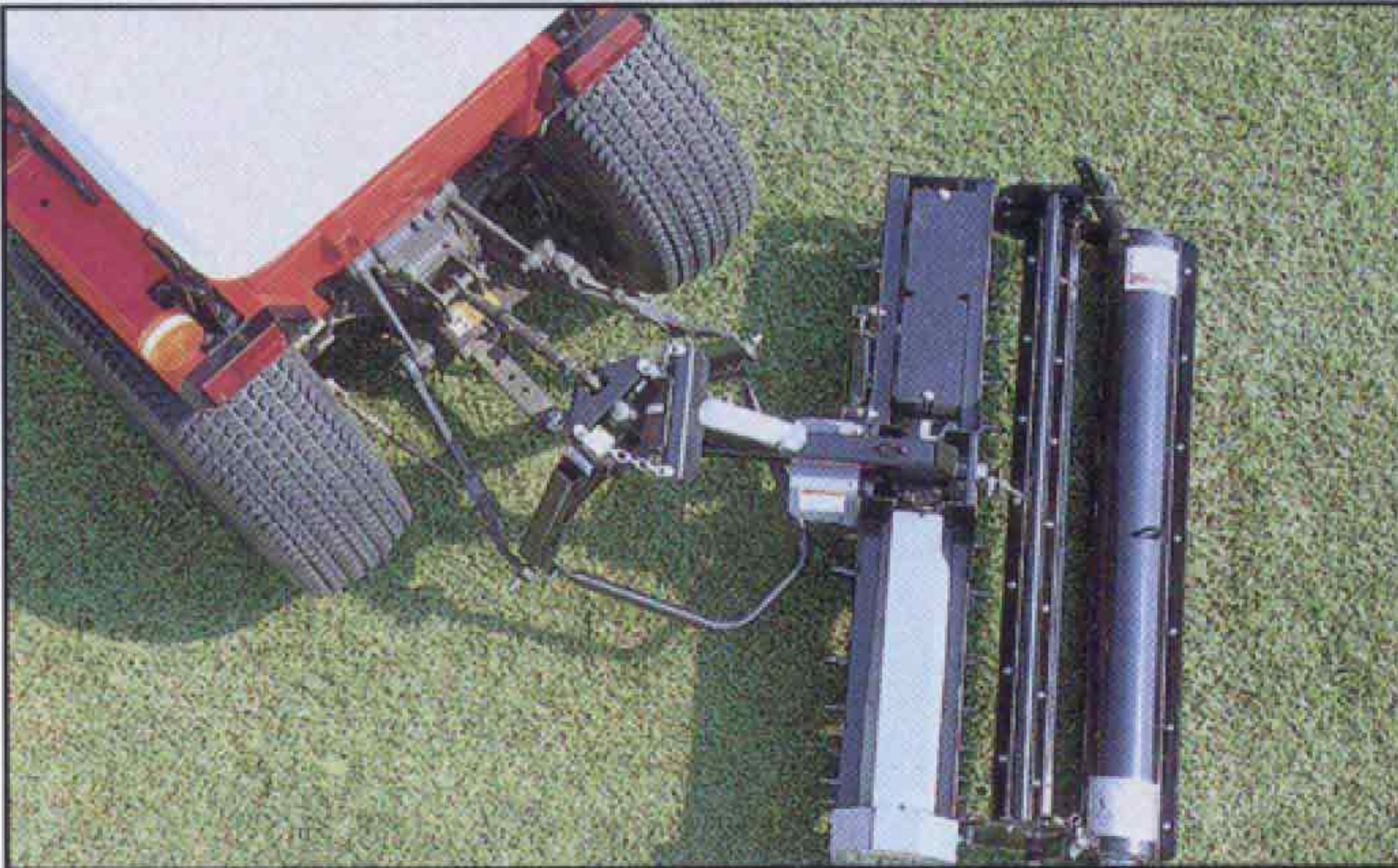
Unique swing hitch allows sharp turns without tearing the established turf.
