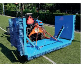
The GKB Brush is the largest brushing machine in the range of GKB. The BR-400 has hydraulically retractable side brushes, so the machine can be easily transported and stored.
