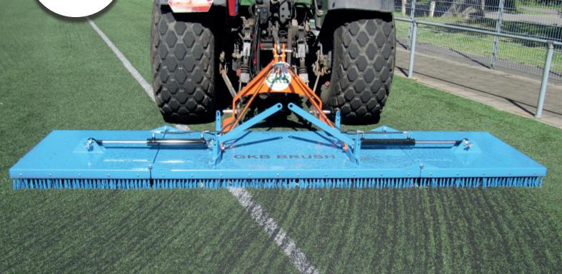
The GKB Brushes were designed with the purpose of brushing artificial turf fast and easy. Brushing artificial turf is an essential part of the weekly maintenance. By using the GKB Brush (BR), Quick-Brush (QB), T-Brush (TB) or Rotobrush (RB) on your sports field, the artificial turf will remain in top-condition.
