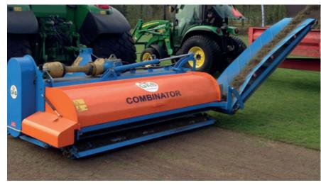
By means of an optional elevator belt the milled or brushed material can be efficiently collected and disposed of or re-used. The elevator belt can be folded away neatly onto the machine for transport & storage. The Combinator is available in four different models.
