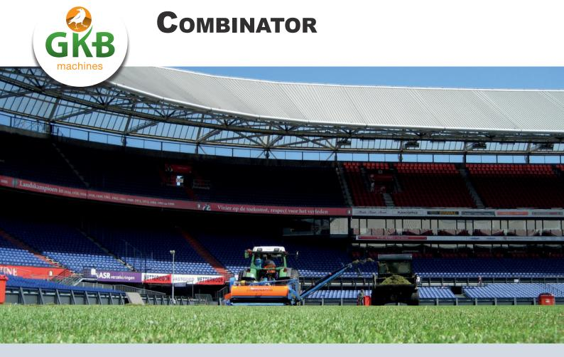
The Combinator has been specially developed for work on grassy areas. The machine can mill to up to 5 cm, making it suitable for both frase mowing and verticutting. The milling is done by means of a special rotor axis equipped with one type of blades. The multifunctional rotor axis is also suitable for scarifying.
