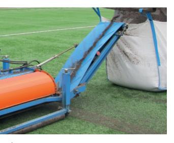
In addition to the use on natural grass, it is also possible to use the Combinator for the removal of infill material on artificial turf. With a special brush the infill material can easily be brushed off of the field.
