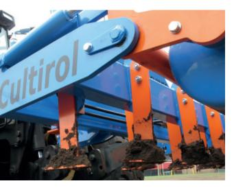
The Cultiriol reworks the soil through breakdown, mixing and levelling. The field can then be seeded with a working depth of 5 to 20 cm. The roller functions as depth control and pressure roller.
