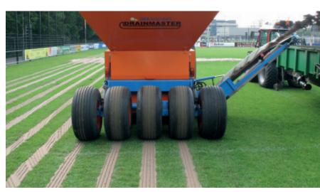
On golf courses and sports fields where surface water is causing a problem, the Drainmaster the solution. The created strands ensure faster drainage which ensures a higher playing capacity. By milling the field it can be perfectly leveled and cleaned if necessary, to keep the system functioning optimally.
