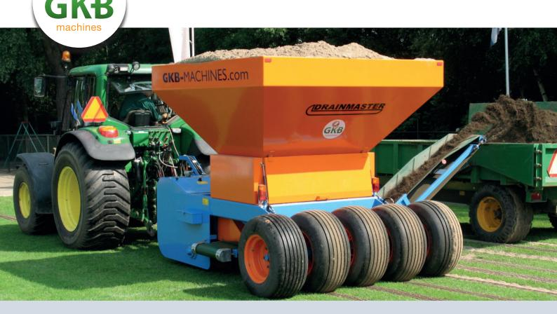
THE GKB DRAINMASTER IS THE PERFECT MACHINE FOR ENSURING EXCELLENT DRAINAGE OF THE TOPSOIL. THE DRAINMASTER ACHIEVES THIS BY DIGGING 2 OR 3 TRENCHES, REMOVING THE SOIL, FILING THE TRENCHES WITH SAND AND THEN COMPACTING THE SAND. THE MILLED SOIL CAN OFTEN BE USED AS A DRESS GROUND.
