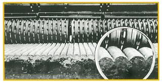
Notice the perfect seedbed. Each seed is deposited at just the right depth where it will germinate quickly. Notched rollers place most of the seed at a depth of 1/2". Seedbed is left smooth and firm, small stones are pressed down.
