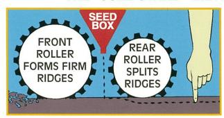
Front rollers crush lumps, press down small stones, and form a firm seedbed. Precision seeding devices meter out the seed onto the well prepared seedbed. Rear rollers split the shallow ridges formed by the front rollers and gently firm the soil around the tiny seeds.
