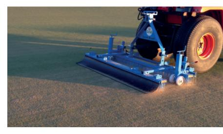
REGULARLY BRUSHING FIELDS PREVENTS IMPAIRED DRAINAGE, DETERIORATING TECHNICAL CHARACTERISTICS BY HARDENING AND THE IMAGE OF A POLLUTED FIELD. THE BRUSHED FIELDS WILL HAVE THE SAME APPEARANCE AS ON THE DAY OF COMMISSIONING.
