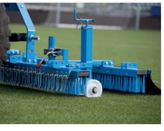
THE GKB QUICK BRUSH CAN BE EQUIPPED WITH MANY EXTRAS. FOR EXAMPLE THE FLIP-OVER TOOL, WHICH IS DESIGNED TO APPLY INFILL MATERIAL TO NEW FIELDS.
