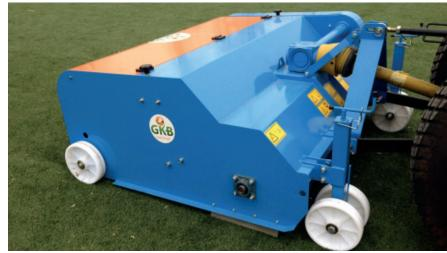
THE LITTERED INFILL MATERIAL IS SWEPT UP BY A DEPTH-ADJUSTABLE BRUSH AND TRANSPORTED TO THE SHAKING SCREEN. THE DIRT MOVES OVER THE SCREEN AND FALLS IN THE WASTE BIN, AND THE FILTERED INFILL MATERIAL FALLS THROUGH THE SCREEN BACK ONTO THE FIELD. AN ADJUSTABLE SUCTION UNIT WITH DISPOSABLE DUST BAGS IS LOCATED ABOVE THE SHAKING SCREEN, TO CLEAR THE AIR OF ANY DUST.
