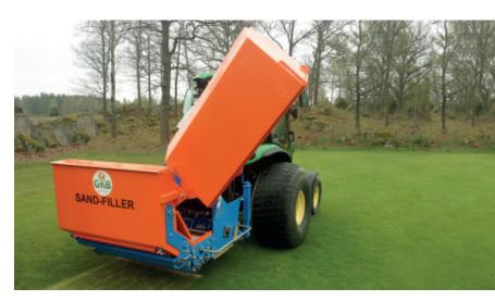
THE DRIED SAND IS DEPOSITED IN THE FUNNEL SHAPED BUNKER. THE SAND INLET IS HYDRAULICALLY CONTROLLED BY AN ADJUSTABLE CONTROL VALVE ON THE SIDE OF THE MACHINE. THE EXCESS MATERIAL, OBTAINED FROM SCARIFYING OR MOWING THE TOP LAYER, IS COLLECTED IN A LATERAL TILTING BIN.
