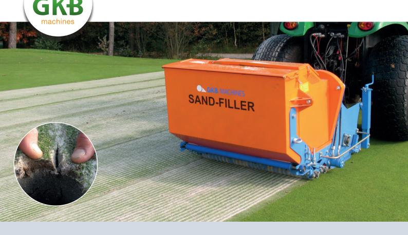
THE SANDFILLER IS DESIGNED TO COUNTER THATCH ON GOLF COURSES AND ESPECIALLY THE GREENS. BECAUSE THE TOP LAYER IS SCARIFIED AND OPTIONALLY FILLED WITH SAND, IT CREATES A GOOD AERATION AND DRAINAGE OF THE FIELD.
