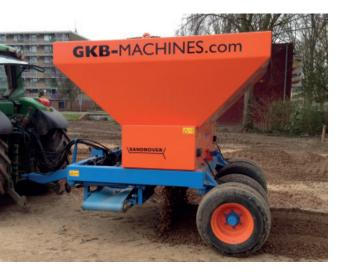
THERE ARE TWO SUBSOILERS LOCATED IN THE BODY, WHICH ASSURE A CONTINUOUS FLOW TO THE DISTRIBUTOR ROLLER. THE FLOW OF SAND IS HYDRAULICALLY TURNED ON AND OFF FROM WITHIN THE TRACTOR, THE THICKNESS OF THE LAYER CAN BE MECHANICALLY SET AT THE BACK OF THE MACHINE.
