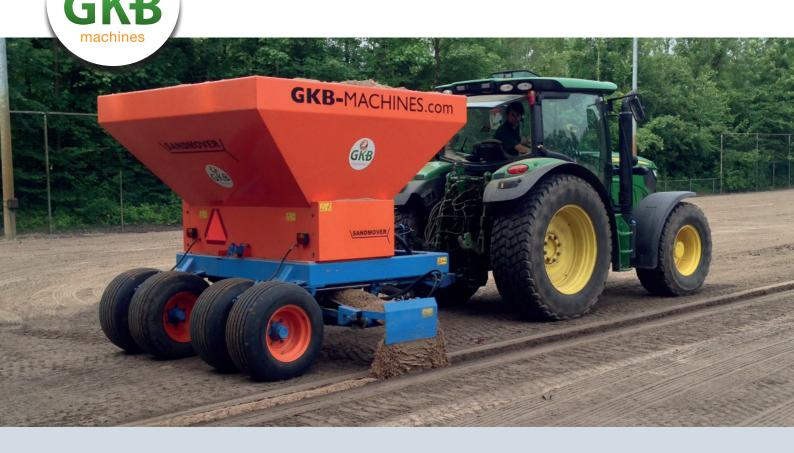
THE SANDMOVER IS THE RIGHT MACHINE FOR QUICKLY ADDING A LAYER OF SAND, SPLIT OR GRAVEL TO THE FIELD. IN ADDITION, THE MACHINE IS SUITABLE FOR FILLING (DRAINAGE) TRENCHES BY THE USE OF A HYDRAULICALLY ADJUSTABLE CONVEYOR BELT.
