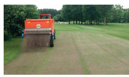
THE MACHINE CAN BE USED ANYWHERE THANKS TO THE FOUR PIVOTING BALLOON TIRES. THESE ENSURE OPTIMUM GROUND PRESSURE SO THAT THE BURDEN ON THE SURFACE IS KEPT TO A MINIMUM.
