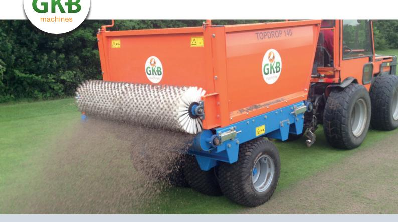
THE GKB TOPDROP IS THE IDEAL MACHINE FOR THE APPLICATION OF TOP LAYERS. THE ROTATING BRUSH DRESSER CAN DISTRIBUTE ALL KINDS OF LOOSE MATERIAL, E.G. SAND, GRAVEL OR RUBBER, ON FIELDS. THE ROTATING BRUSH IS HYDRAULICALLY DRIVEN AND IS EASILY ADJUSTABLE IN SPEED.
