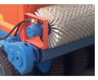
BY ADJUSTING THE BRUSH SPEED FROM WITHIN THE TRACTOR AND ADJUSTING THE MECHANICAL METERING VALVE, THE LAYER THICKNESS CAN BE DETERMINED PRECISELY.
