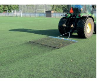
DRAGGING PERPENDICULAR TO THE SWEEPING DIRECTION THE INFILL MATERIAL IS SWEPT INTO THE MAT. DIRT IN THE FORM OF CIGARETTE BUTTS, LEAVES AND SMALL TWIGS WILL BE SWEPT UP DURING TOWING, AND CAN BE EASILY COLLECTED AFTERWARDS.
