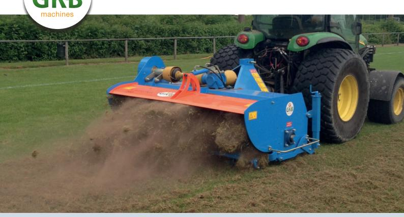
THE GKB VSTRONG HAS BEEN DEVELOPED, BECAUSE OF INCREASING MARKET DEMAND, FOR AN AGGRESSIVE AERATING MACHINE TO REMOVE THATCH. BY REMOVING THATCH, MOSS AND OTHER MATERIAL THE GRASS IS ALLOWED MORE SPACE TO GROW, PROVIDES PERMEABILITY OF THE TOP LAYER, AND INCREASES RESISTANCE TO DISEASE AND INSECTS. IN ADDITION, THE WATER PERMEABILITY OF THE TOP LAYER IS DRASTICALLY IMPROVED.
