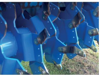
THE VSTRONG USES THE COMBI-ROTOR SYSTEM, WHICH CAN BE USED FOR BOTH TOTAL REMOVAL, WITH THE FRASING BLADES, AS WELL AS VERTICUTTING.
