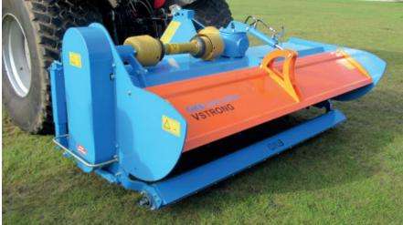
The Vstrong is equipped with an adjustable hydraulic tailgate to guide the output of the dispatched material. The plastic scrapers on the rollers ensure that the rollers always remain clean.
